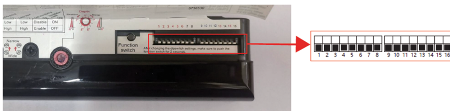
DIP Switch adjustment for Inside sensor
