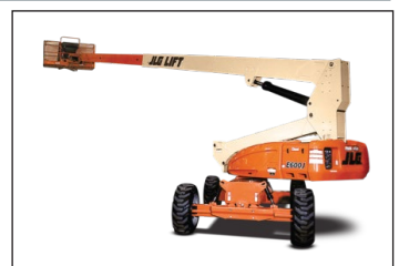
Electric Straight Boom Lifts Platform Height Range : 18.36m - 18.39m Outreach Range : 13.19m - 13.54m
