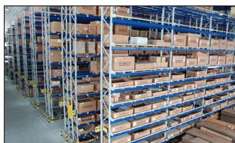
Selective Pallet Racking
